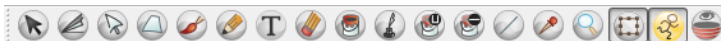
The Flat Tool Toolbar preference expands the toolbar so there are no nested toolsets.
