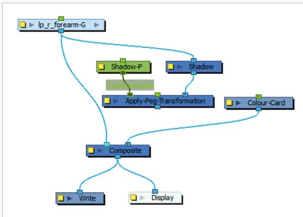
6. Connect the output port of the Apply-Peg-Transformation node to your scene's main composite, just right of the connection for your character rig. This way, the shadow will appear behind your character rig.
